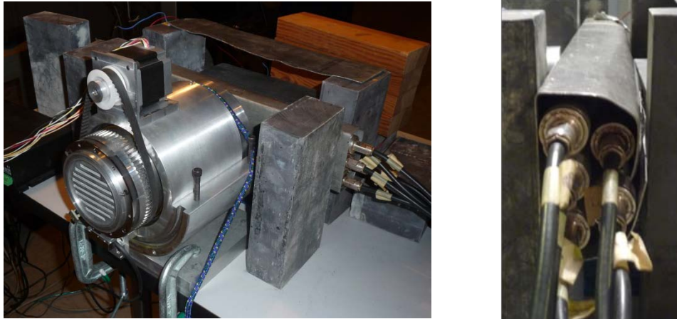
Figure 14: RMC Configured with Combined Detectors. On the left: The detectors were placed sideways to avoid the potential loss of efficiency due to the guard rings. On the right: The detectors were lined up and wrapped in cadmium. They were covered in cadmium, except for an unseen hole behind the masks, to reduce the background thermal neutron counts.
